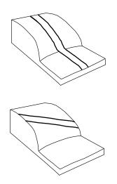
Figure 6: Parallel-Slope (above) and Cross-Slope (below) roads.
