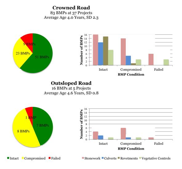
Figure 11: BMP condition grouped by road surface crown or tilt.
